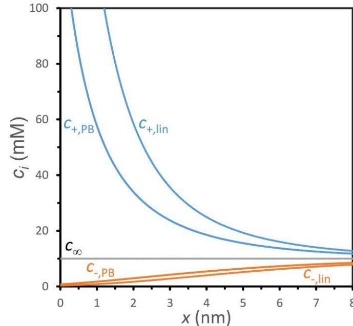
Ion concentration for GCS model (denoted by PB) and a linearized solution (Biesheuvel, 2020)
