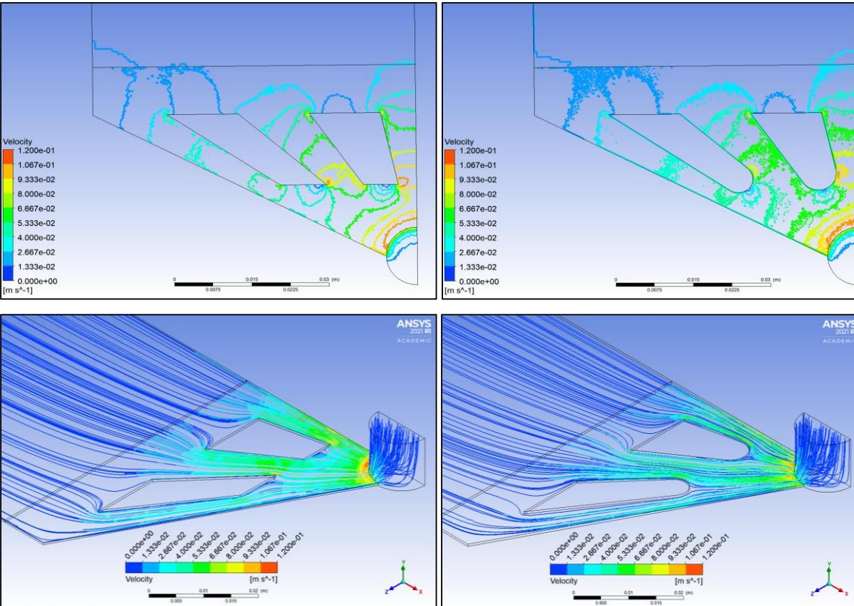
Isotaches (top) and velocity track (bottom) for standard diffusor shape (left) and optimized geometry (right) (Franz, 2021)
