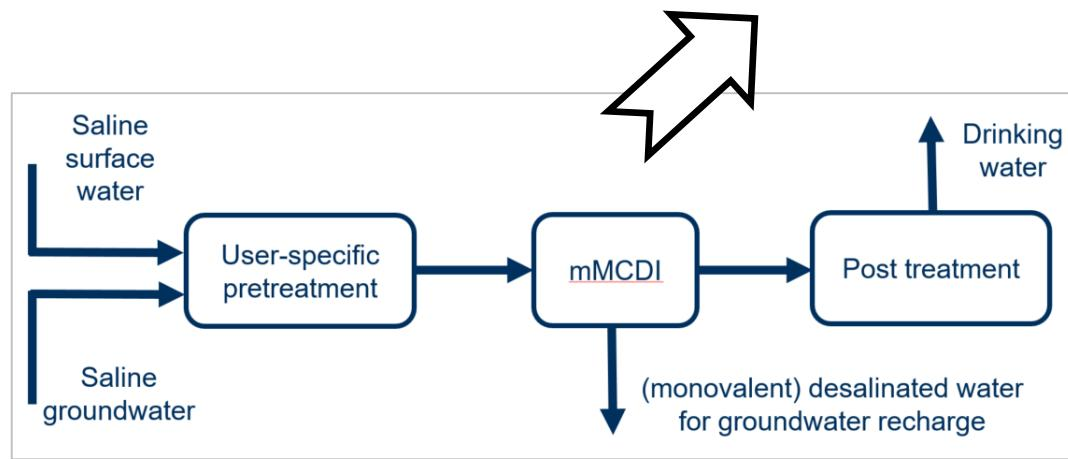
Process principle for implementation of mMCDI (monoselective membrane capacitive deionization) in desalination of saline waters
